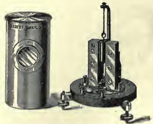
FIG. 2.—Movable Coil Galvanometer.
